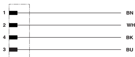
Contact assignment of the M8 plug
