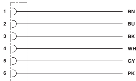
Contact assignment of the DEUTSCH DT06-6S
