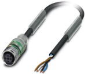
Sensor/actuator cable, 4-position, PVC, black RAL 9005, free cable end, on Socket straight M12, A-coded, with 2 LEDs, cable length: 1.5 m
