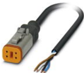
Sensor/actuator cable, 4-position, PUR halogen-free, black-gray RAL 7021, free cable end, on Socket straight DEUTSCH DT06-4S Clip locking, cable length: 5 m
