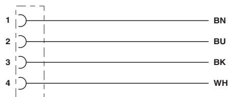
Contact assignment of the DEUTSCH DT06-4S
