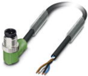
Sensor/actuator cable, 4-position, PVC, black RAL 9005, Plug angled M12, A-coded, on free cable end, cable length: 10 m
