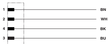
Contact assignment of the M12 plug
