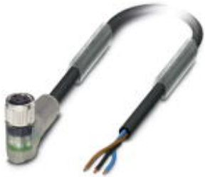
Sensor/actuator cable, 3-position, PVC, black RAL 9005, free cable end, on Socket angled M8, with 2 LEDs, cable length: 5 m
