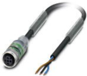
Sensor/actuator cable, 3-position, PVC, black RAL 9005, free cable end, on Socket straight M12, A-coded, with 2 LEDs, cable length: 1.5 m
