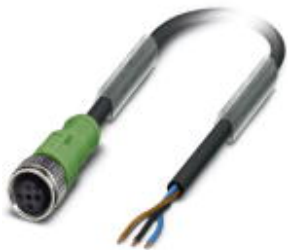
Sensor/actuator cable, 3-position, PVC, black RAL 9005, free cable end, on Socket straight M12, A-coded, cable length: 5 m
