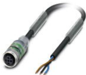
Sensor/actuator cable, 3-position, PVC, black RAL 9005, free cable end, on Socket straight M12, A-coded, with 2 LEDs, cable length: 3 m
