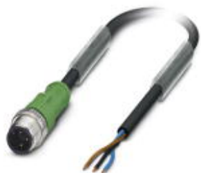
Sensor/actuator cable, 3-position, PVC, black RAL 9005, Plug straight M12, A-coded, on free cable end, cable length: 1.5 m
