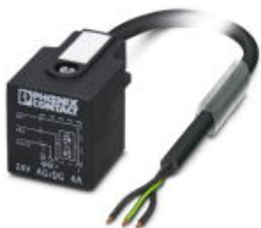
Sensor/actuator cable, 3-position, PUR/PVC, black RAL 9005, free cable end, on Valve connector A, with 1 LED, cable length: 5 m
