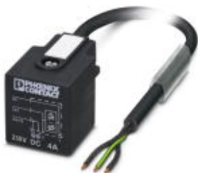
Sensor/actuator cable, 3-position, PVC, black, free cable end, on Valve connector A, with 1 LED, connected with Varistor, cable length: 3 m
