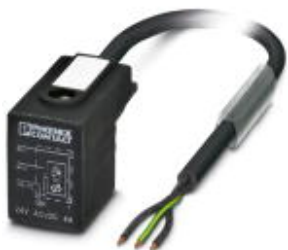
Sensor/actuator cable, 3-position, PVC, black RAL 9005, free cable end, on Valve connector B (10 mm), with 1 LED, connected with Varistor, cable length: 1.5 m
