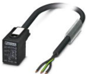
Sensor/actuator cable, 3-position, PVC, black RAL 9005, free cable end, on Valve connector B (10 mm), with 1 LED, connected with Z diode, cable length: 1.5 m
