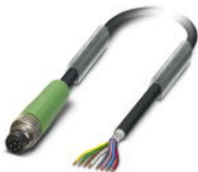
Sensor/actuator cable, 8-position, PUR halogen-free, black RAL 9005, shielded, Plug straight M8, on free cable end, cable length: 1.5 m
