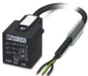
Sensor/actuator cable, 3-position, PVC, black RAL 9005, free cable end, on Valve connector A, with 1 LED, connected with Varistor, cable length: 1.5 m
