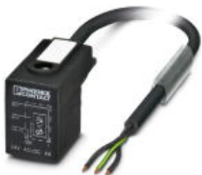
Sensor/actuator cable, 3-position, PVC, black RAL 9005, free cable end, on Valve connector BI (11 mm), with 1 LED, connected with Varistor, cable length: 1.5 m
