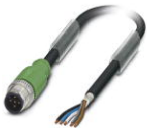
Sensor/actuator cable, 5-position, PUR halogen-free, black-gray RAL 7021, shielded, Plug straight M12, A-coded, on free cable end, cable length: 30 m
