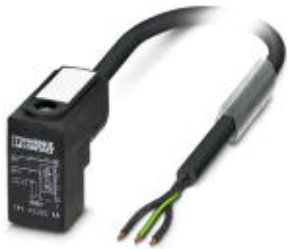
Sensor/actuator cable, 3-position, PVC, black RAL 9005, free cable end, on Valve connector C (8 mm), with 1 LED, connected with Z diode, connected with Z diode, cable length: 5 m
