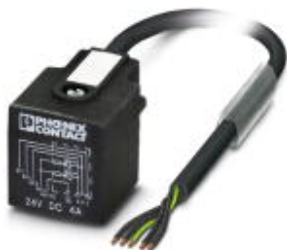
Sensor/actuator cable, 5-position, PVC, black, free cable end, on Valve connector AD (pressure switch), with 2 LEDs, cable length: 5 m
