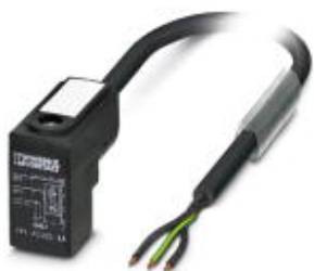
Sensor/actuator cable, 3-position, PVC, black RAL 9005, free cable end, on Valve connector CI (9.4 mm), with 1 LED, connected with Z diode, cable length: 5 m
