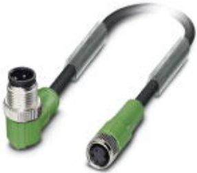
Sensor/actuator cable, 3-position, PUR halogen-free, black-gray RAL 7021, Plug angled M12, A-coded, on Socket straight M8, cable length: 5 m
