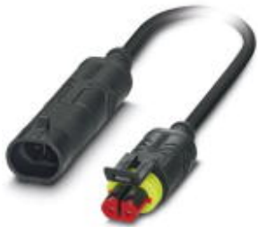
Sensor/actuator cable, 2-position, PUR halogen-free, black-gray RAL 7021, Plug straight Superseal Clip locking, on Socket straight Superseal Clip locking, cable length: 0.6 m
