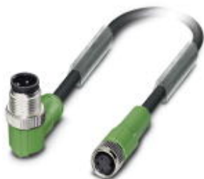
Sensor/actuator cable, 3-position, PUR halogen-free, black-gray RAL 7021, Plug angled M12, A-coded, on Socket straight M8, cable length: 10 m
