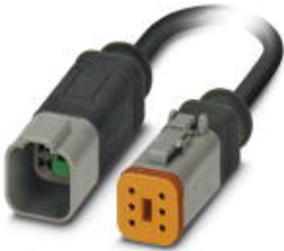
Sensor/actuator cable, 6-position, PUR halogen-free, black-gray RAL 7021, Plug straight DEUTSCH DT04-6P Clip locking, on Socket straight DEUTSCH DT06-6S Clip locking, cable length: 0.6 m
