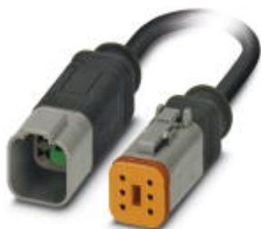
Sensor/actuator cable, 6-position, PUR halogen-free, black-gray RAL 7021, Plug straight DEUTSCH DT04-6P Clip locking, on Socket straight DEUTSCH DT06-6S Clip locking, cable length: 3 m
