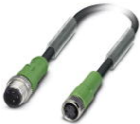
Sensor/actuator cable, 3-position, PVC, black RAL 9005, Plug straight M12, A-coded, on Socket straight M8, cable length: 0.3 m
