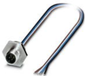
Sensor/actuator flush-type plug, 4-pos., M12, A-coded, front/screw mounting with M20 x 1.5 thread, with 0.5 m TPE litz wire, 4 x 0.34 mm 2 , brass housing
