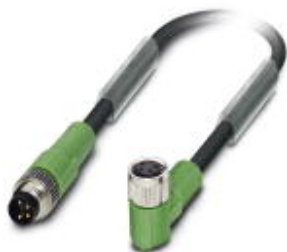
Sensor/actuator cable, 4-position, PVC, black RAL 9005, Plug straight M8, on Socket angled M8, cable length: 0.3 m
