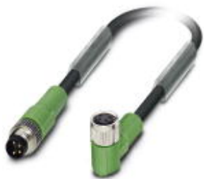
Sensor/actuator cable, 4-position, PVC, black RAL 9005, Plug straight M8, on Socket angled M8, cable length: 1.5 m
