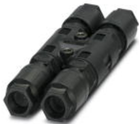
QUICKON H-distributor, black, 4 pos. +PE, 1.0 mm 2 ... 2.5 mm 2 / 690 V / 20 A, for cable diameters of 6 mm ... 11 mm, with a sealing bolt.
