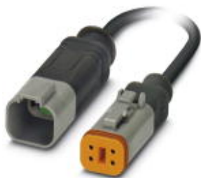
Sensor/actuator cable, 4-position, PUR halogen-free, black-gray RAL 7021, Plug straight DEUTSCH DT04-4P Clip locking, on Socket straight DEUTSCH DT06-4S Clip locking, cable length: 1.5 m
