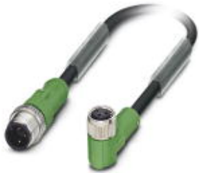
Sensor/actuator cable, 3-position, PVC, black RAL 9005, Plug straight M12, A-coded, on Socket angled M8, cable length: 3 m
