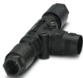
QUICKON T-distributor, black, 4+PE-pos., 1.0 mm² ... 2.5 mm²/690 V/20 A, for cable diameter of 6 mm ... 11 mm, with two QUICKON nuts
