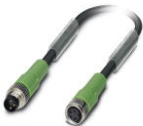
Sensor/actuator cable, 3-position, PUR halogen-free, black-gray RAL 7021, Plug straight M8, on Socket straight M8, cable length: 0.5 m
