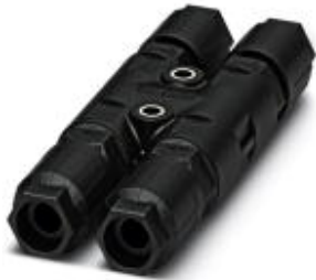
H distributor, QUICKON connection, number of positions: 2+PE, 0.5 mm 2 ... 1.5 mm 2 , 690 V, 17.5 A, black, with QUICKON nut, cable diameter range: 10 mm ... 13 mm, with a sealing bolt
