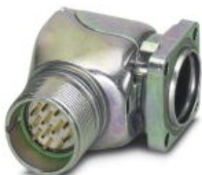
Device connector, front mounting, angled rotatable, Screw locking, M23, number of positions: 12, type of contact: Pin, Solder connection, Axial O-ring, 4x Ø 3.2, shielded: yes
