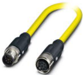
Sensor/actuator cable, 8-position, PVC, yellow, shielded, Plug straight M12 SPEEDCON, A-coded, on Socket straight M12 SPEEDCON, A-coded, cable length: 15 m
