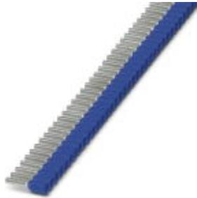
Taped ferrules, 0.75 mm<sup>2</sup>, sleeve length: 8 mm, with plastic collars, according to DIN 46228-4, special color: blue according to NF C63-023, with function end for safe and convenient processing with the Crimphandy, 20 strips each with 50 sleeves per strip.
