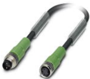
Sensor/actuator cable, 3-position, PVC, black RAL 9005, Plug straight M8, on Socket straight M8, cable length: 5 m
