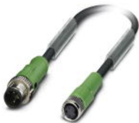
Sensor/actuator cable, 3-position, PUR halogen-free, black-gray RAL 7021, Plug straight M12 SPEEDCON, A-coded, on Socket straight M8, cable length: 0.6 m
