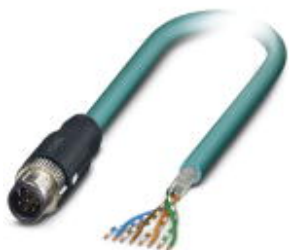
Network cable, Ethernet CAT5 (1 Gbps), 8-position, PUR, water blue RAL 5021, shielded, Plug straight M12 SPEEDCON / IP67, coding: A, on free cable end, cable length: 10 m
