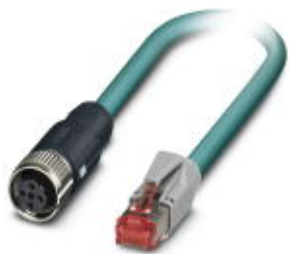
Network cable, Ethernet CAT5 (100 Mbps), 4-position, PUR, water blue RAL 5021, shielded, Plug straight RJ45 / IP20, on Socket straight M12 SPEEDCON / IP67, coding: D, cable length: 5 m
