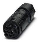
Circular connectors (cable-side), Connector, color: black, number of positions: 5, Min. wire cross section: 1.5 mm<sup>2</sup>, Max. conductor cross section: 6 mm<sup>2</sup>, nom. voltage: 690 V AC, Rated current: 35 A, Connection method: Screw connection, Type of contact: Pin, Min. cable diameter: 8 mm, Max. cable diameter: 12 mm
