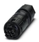
Circular connectors (cable-side), Connector, color: black, number of positions: 5, Min. wire cross section: 1.5 mm², Max. conductor cross section: 6 mm², nom. voltage: 690 V AC, Rated current: 35 A, Connection method: Screw connection, Type of contact: Pin, Min. cable diameter: 16 mm, Max. cable diameter: 21 mm
