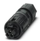
Circular connectors (cable-side), Connector, color: black, number of positions: 3, Min. wire cross section: 1.5 mm², Max. conductor cross section: 6 mm², nom. voltage: 690 V AC, Rated current: 35 A, Connection method: Screw connection, Type of contact: Pin, Min. cable diameter: 12 mm, Max. cable diameter: 16 mm
