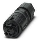
Circular connectors (cable-side), Connector, color: black, number of positions: 3, Min. wire cross section: 1.5 mm<sup>2</sup>, Max. conductor cross section: 6 mm<sup>2</sup>, nom. voltage: 690 V AC, Rated current: 35 A, Connection method: Screw connection, Type of contact: Pin, Min. cable diameter: 8 mm, Max. cable diameter: 12 mm
