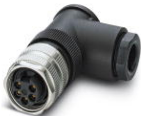
Connector, 5-position, Socket angled 7/8"-16UNF, Screw connection, knurl material: Zinc die-cast, nickel-plated, cable gland Pg13,5, external cable diameter 10 mm ... 12 mm
