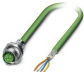
Bus system flush-type socket, PROFINET, 4-pos., M12, shielded, D-coded, SPEEDCON, rear/screw mounting with Pg9 thread, with 5.0 m bus cable, 2 x 2 x 0.34 mm 2
